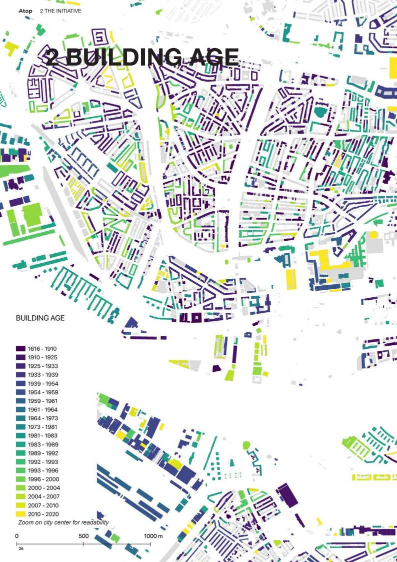
The date of construction of a building is a good indicator to assess its structural system. Buildings which have been build too recent have their structures too much optimized to have more weight added, buildings which have been build too long ago have weaker structures. Based on structural analysis run in collaboration with a civil engineer, buildings built in the Netherlands between 1900 and 1990 can be considered to host a vertical extension.
